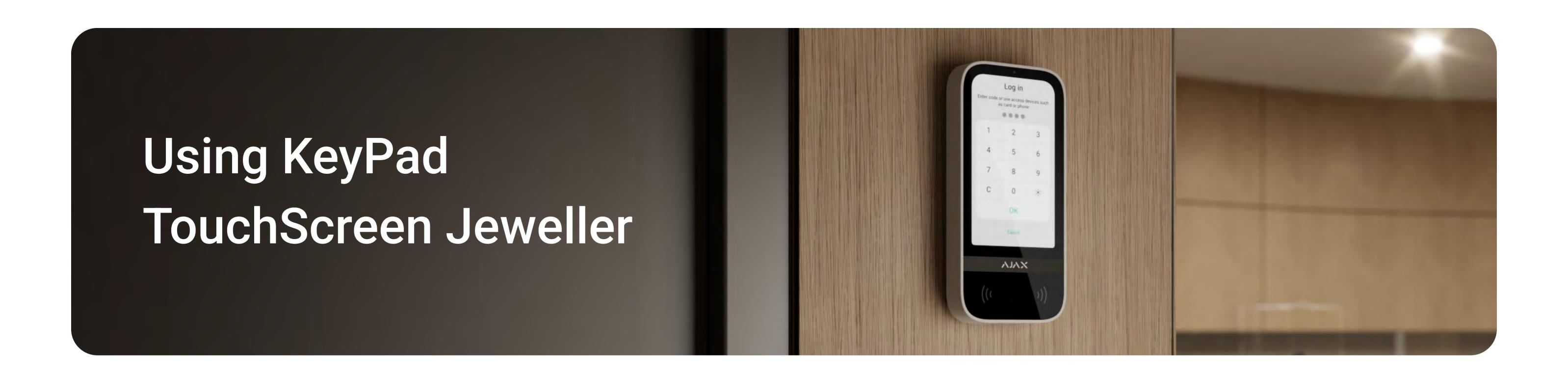
**KeyPad TouchScreen Jeweller** is a wireless keypad with a touch screen designed for managing the Ajax security system. Users can authenticate using smartphones, Tag key fobs, Pass cards, and codes. The device is intended for indoor use. KeyPad TouchScreen Jeweller is protected against attempts to guess the code and can raise a silent alarm when the code is entered under duress.
