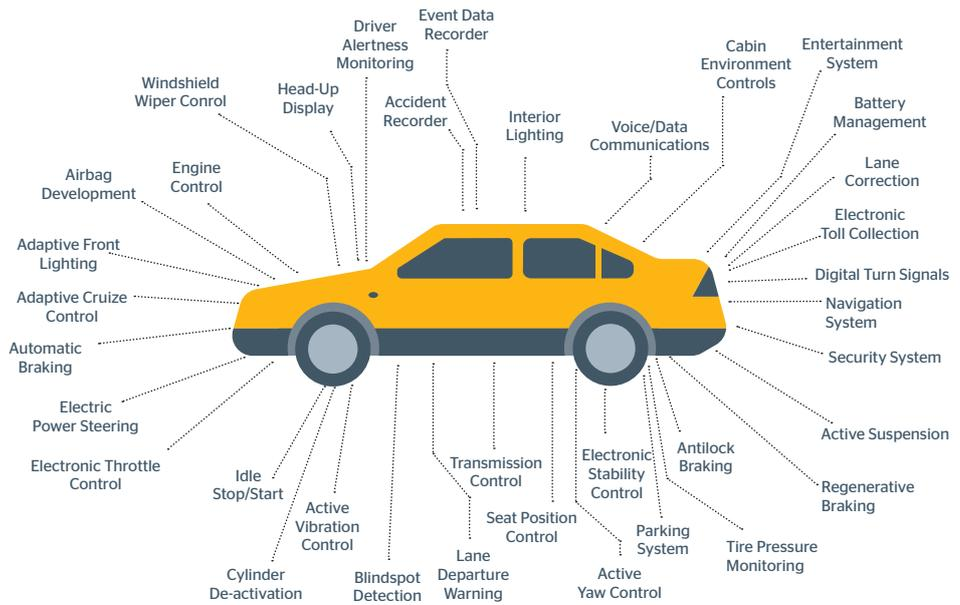
Figure 1: Sources of vehicle-generated data<sup>3</sup>
