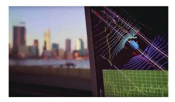
RAC's Intellibus also uses its 3D and 2D LiDARs as well as the stereovision cameras to detect obstacles movement and changes to the traffic environment.
